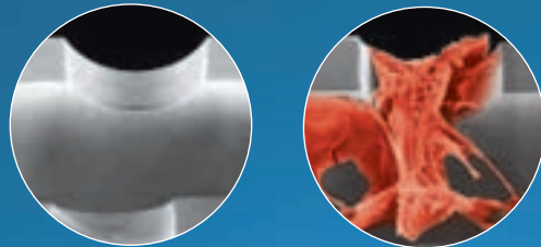
Uncoated catheter exhibits large thrombus growing through the catheter side hole, while the coated surface remains clean. Image colorized to show detail.
