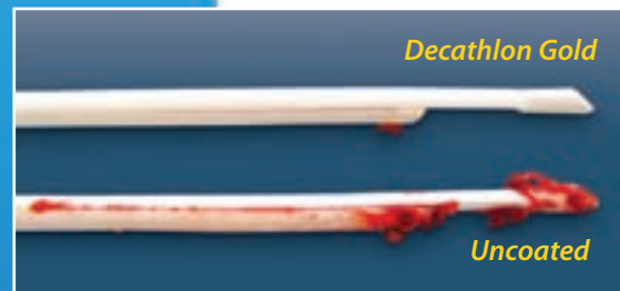
In-vitro blood loop thromboresistance test shows a 96% reduction in thrombus accumulation on the Decathlon Gold catheter.
